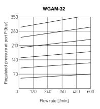
5 MINIMUM PRESSURE VERSUS FLOW DIAGRAMS based on mineral oil ISO VG 46 at 50°C
