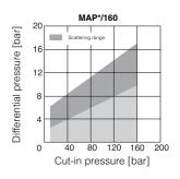
The graphs show, according to the set cut-in pressure, the pressure difference between the insert and the resting positions of the pressure switch electric
