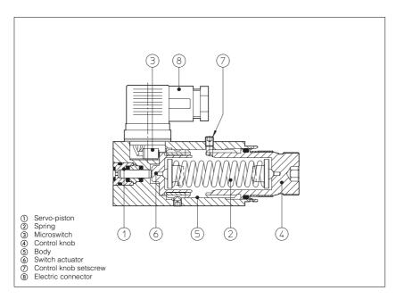
WMAP are pressure switches when open or close an electrical contact when the pressure in the hydrau-lic circuit reaches a given setting.
