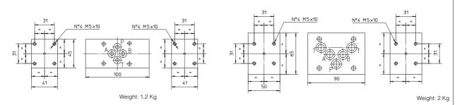
For versions 11 and 13 the pressure switch is mounted on side of port A. For version 14 the pressure switch is mounted on side of port B. For versions 12, 17, 18 the pressure switch is mounted on both sides.
